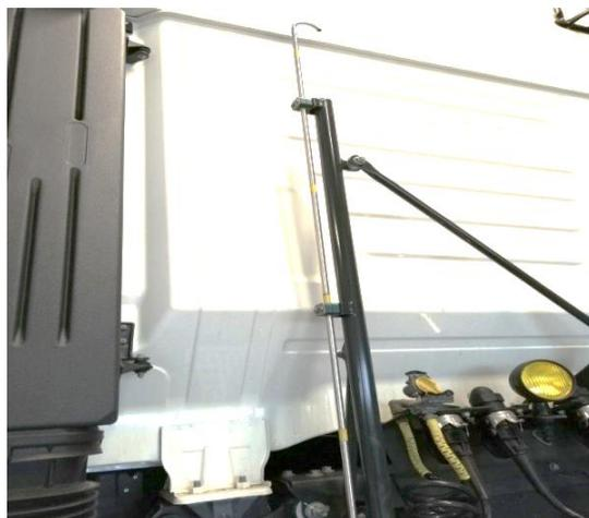
Figure 5-1: Blow-off lance behind the driver's cab; source: ZDK
