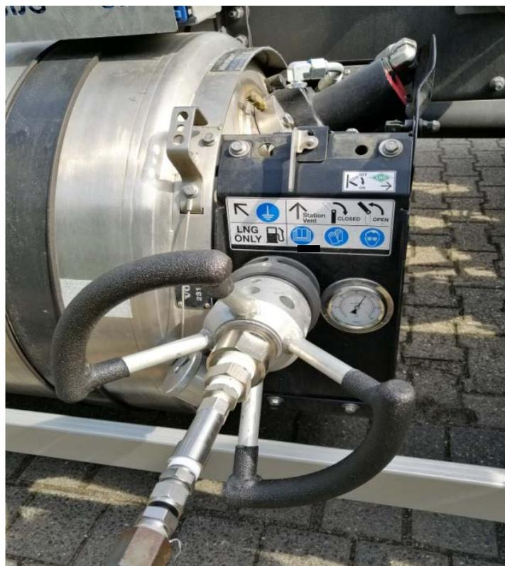
Figure 6-7: Connection of the blow-off device; source: ZDK
