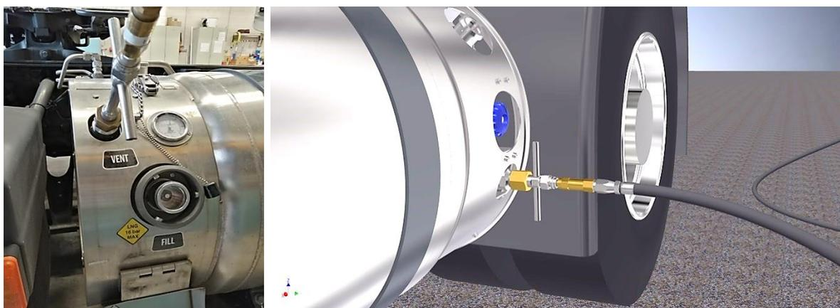
Figure 6-2: Installed blow-off device chart LNG tank (attached); source: ZDK (left figure)/GasCom (right figure)
