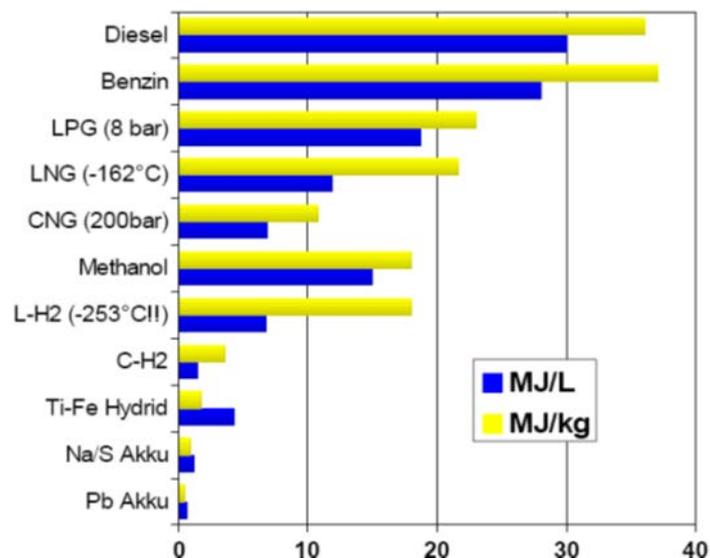
Figure 4-1: Energy density incl. storage medium (tank);
