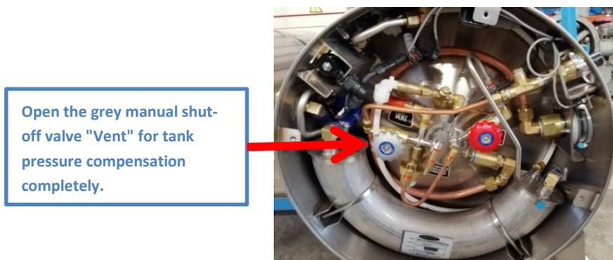
Figure 6-3: Grey manual shut-off valve "Vent"; source: ZDK
