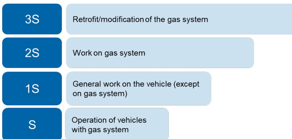
Figure 3-1: Qualification levels for work on gas vehicles
