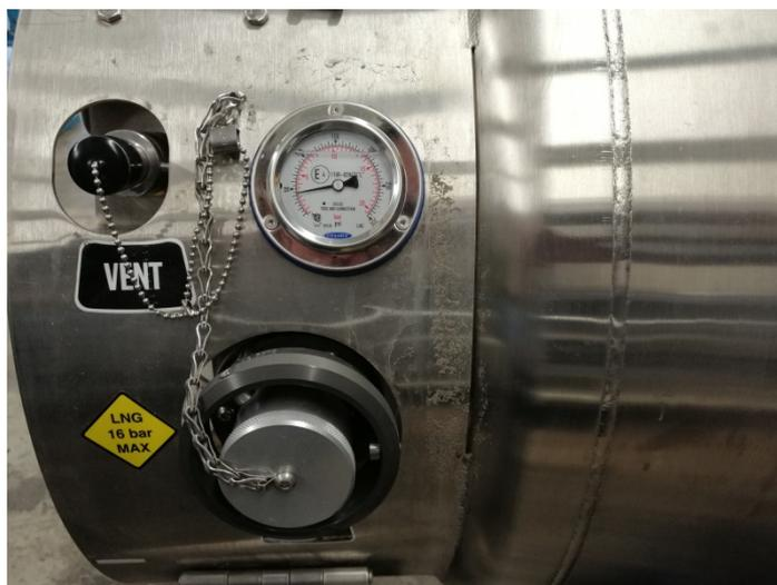
Figure 4-3: LNG tank (cryotank); source: ZDK
