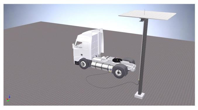
Figure 6-1: Connection diagram "Blow-off device and canopy chimney"; source: GasCom
