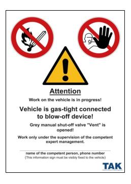
Figure 6-4: Identification of vehicles with LNG drive in the workshop; source: ZDK
