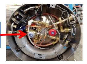
Figure 6-3: Grey manual shut-off valve "Vent"; source: ZDK
