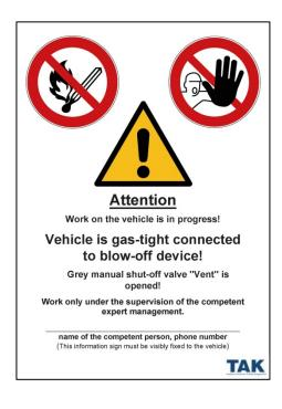
Figure 6-9: Identification of vehicles with LNG drive in the workshop; source: ZDK
