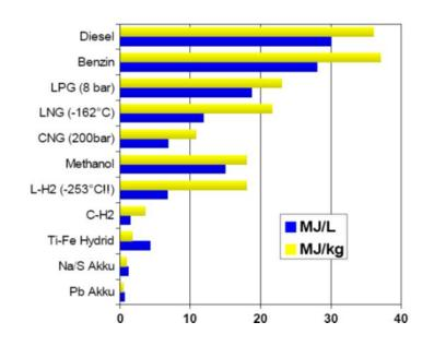
Figure 4-1: Energy density incl. storage medium (tank); source: Daimler AG - Research and Technology
