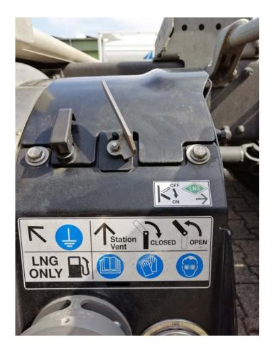
Figure 6-8: "Station Vent" - valve on the tank; source: ZDK
